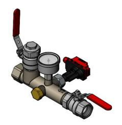
Installation: Screw the flow switch into the appropriate size Applications Engineering Valve Set or CPVC Tee piece with adaptor as shown above with the ¾" BSP Female thread on the flow switch screwing into the ¾" Male thread.
