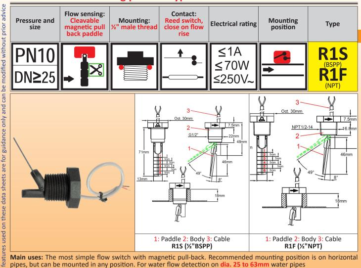
Main uses: The most simple flow switch with magnetic pull-back. Recommended mounting position is on horizontal pipes, but can be mounted in any position. For water flow detection on dia. 25 to 63mm water pipes **Functional principle:**
