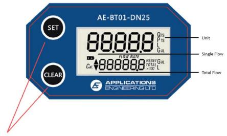
Set Key: Switch interface between flow rate and total flow
