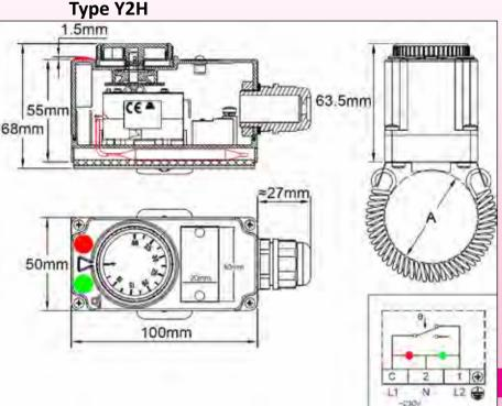
Housing: IP65, 100 x 50 x 75 mm, PC-ABS, 20%FG, UL94V0. High impact and UV resistance, with silicone waterproof gasket on thermostat shaft.
